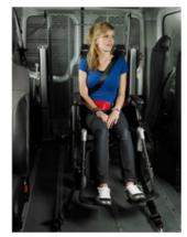
Meanwhile, the PROTEKTOR® system provides critical stabilization for passengers in the event of a collision. The design rules out any possibility of the wheelchair being improperly secured. The pelvic belt ensures that the passenger is always secure.
